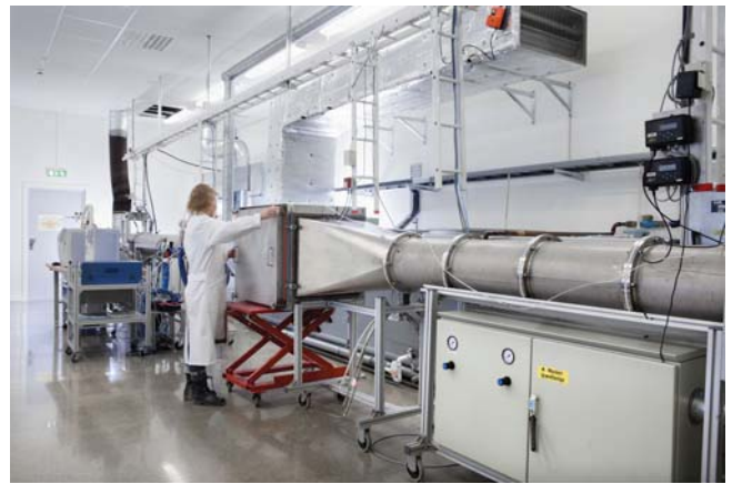
Filter test rig in Camfil Tech Center, Sweden
